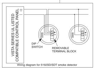
14 to 22 gauge wire to provide easy wiring connections. The detectors are designed to meet all applicable requirements for UL Commercial and Residential Fire installations as well as NFPA 72 requirements when installed in compliance with the National Electric Code and approved/listed control panels.
