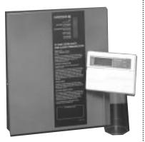
5110XM...The industry's most flexible control for slave or standalone dual digital communication. The 5110XM is a UL Listed, microprocessor based fire alarm control/communicator that supports five hardwired zones. It may be used as a slave Digital Alarm Communicator Transmitter (DACT) providing central or remote station service for a central or remote station listed Fire Alarm Control Panel (FACP). It may also be used as a stand alone non-coded local, central station or remote station control.
